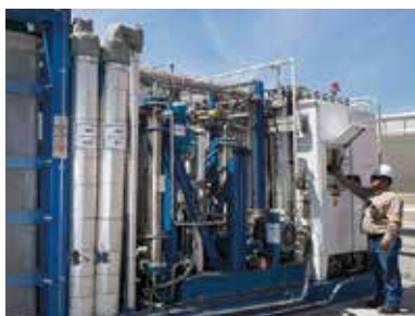
HYOS-R — state-of-the-art mid-range on-site hydrogen generator via steam reforming
